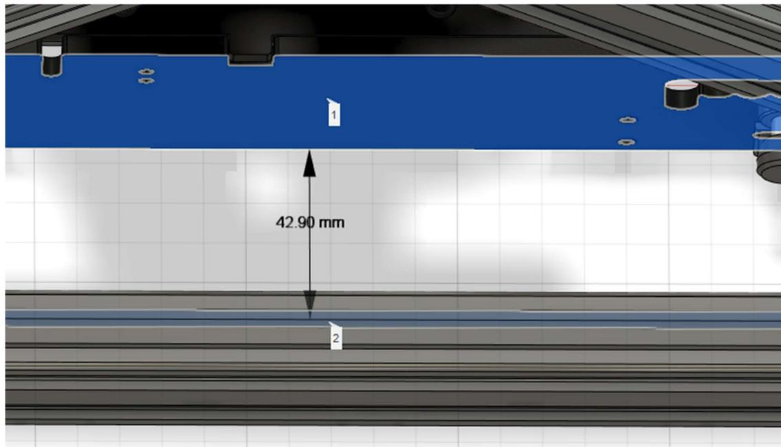
The length of the belt can vary, so the tensioning rods do not necessarily have to be placed in the same position as on the old belt.
