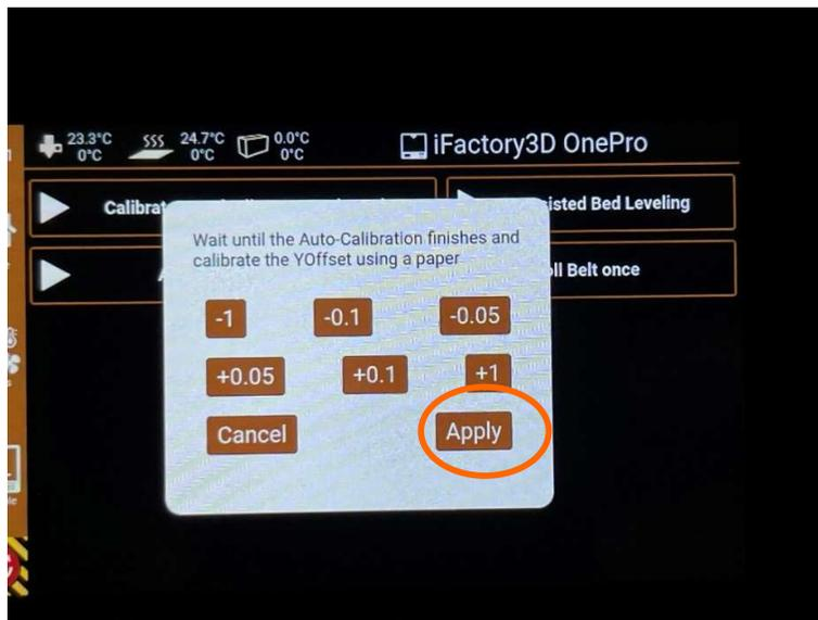
**After the calibration process, Y-hardstops must be mounted in Y0-Position to prevent damage to the print bed in case of printing issues.**
