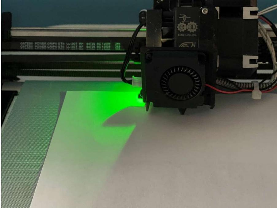
Now move the printhead down in [-1], later in smaller increments, until the nozzle scratches the paper. To do this, move the paper slightly back and forth under the nozzle and check whether slight marks appear. Then confirm the setting with "Apply".
