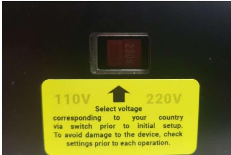
**Note:** Labelling can be different for each machine. "110V" supports all voltages from 100V up to 120V [US standard], while "220V" supports all voltages from 220V up to 240V [EU standard].
