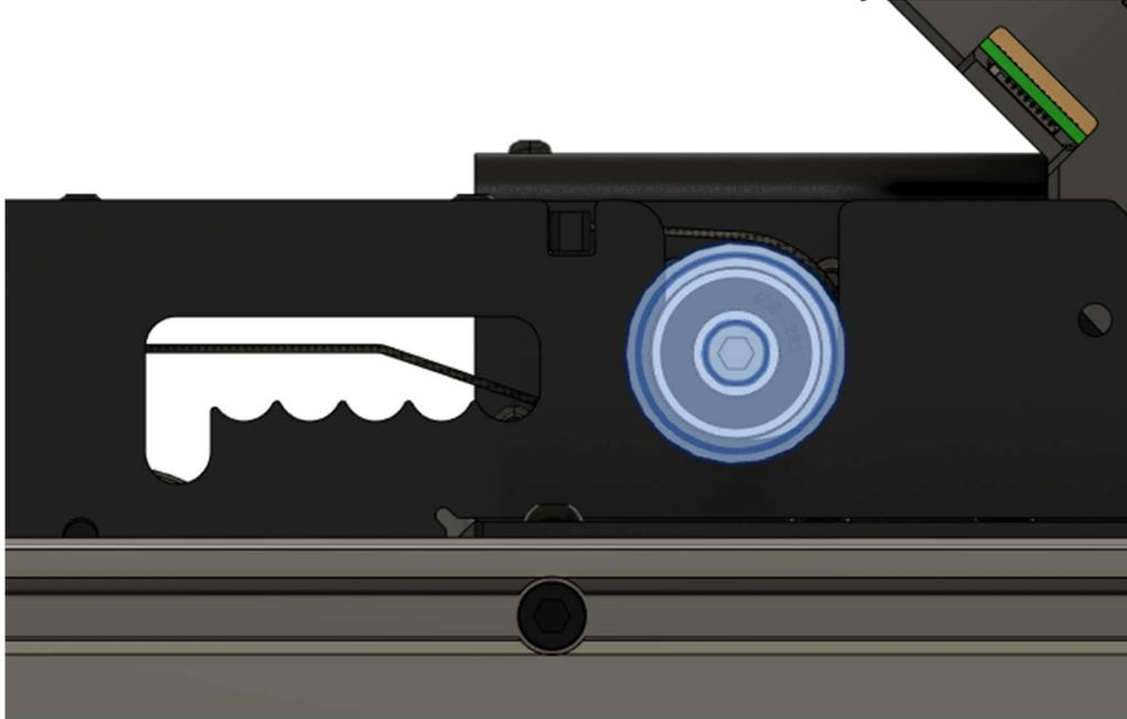
Half of the coupler for the Z-motor should be still connected to the front roll.
