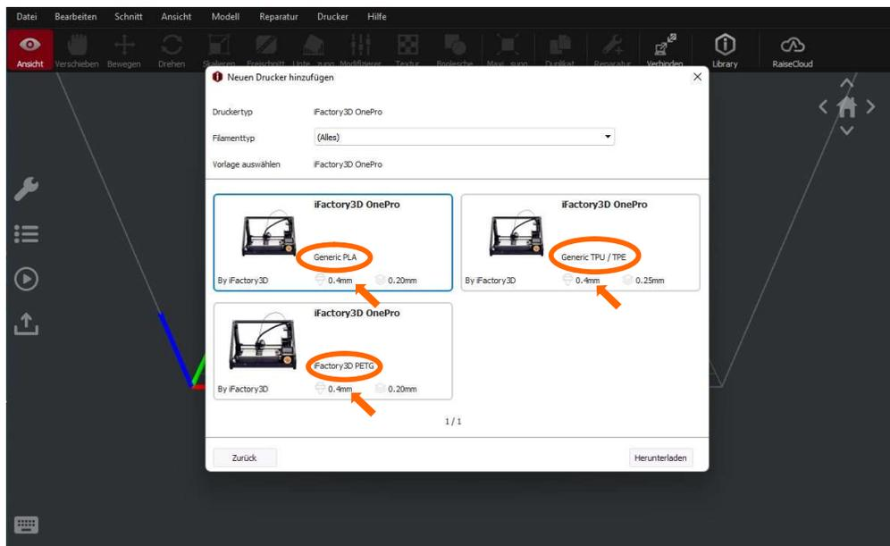
Prefabricated standard profiles can be found here, which may still need to be slightly adapted to the material and/or nozzle diameter you plan on using.
