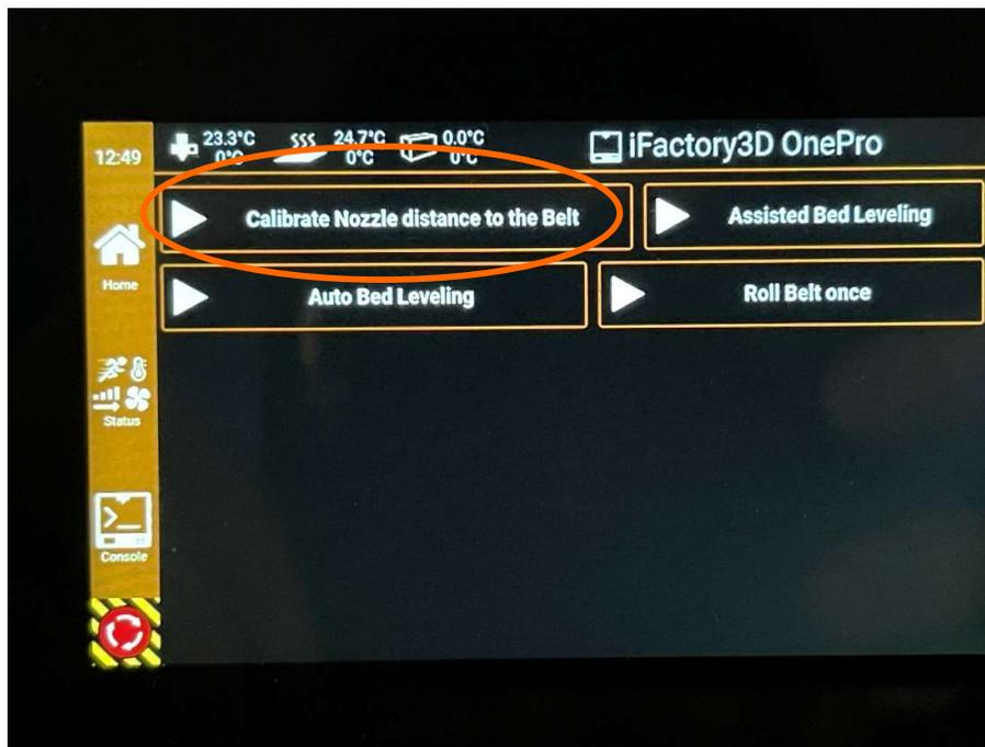
Now calibrate the distance between the nozzle and the print bed using a piece of paper. To do this, select "Calibrate nozzle distance to the belt" via the menu.
