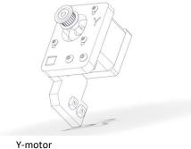
Slide the X and Y motors on the top 20x20x530 extrusion until the T-nuts from the motorbracket hit the channel of the 20x20x460 extrusion.
