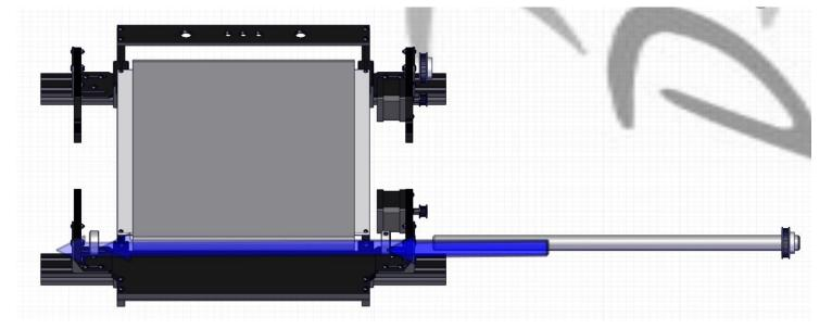
Now push the 20mm shafts into the front bearings and through the belt. Start from the right side.
