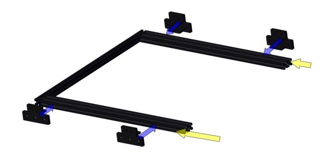
20x20 extrusion and 40x20 extrusions
