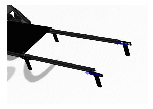
Put a silicon spacer in every countersink of the new 20x20 profiles.
